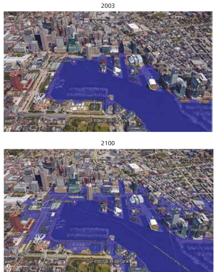
Figure 11. The combined effect of sea-level rise and increased storm surge on inundation from a Hurricane Isabel-like storm in 2100, under the Growing Emissions pathway, compared to 2003.
